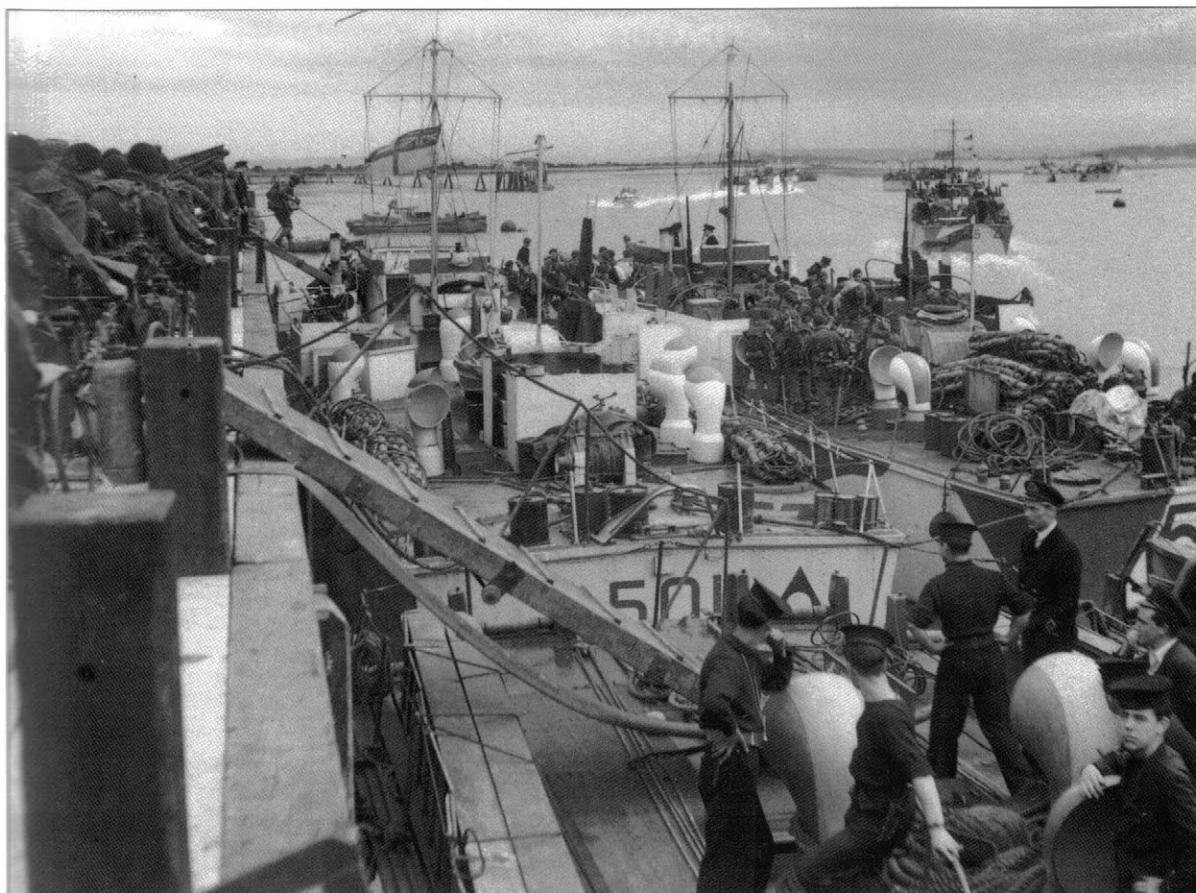
Commandos from 1st Special Service Brigade embark onto LCI (S) - Landing Craft Infantry Small - at Warsash in Southampton Water. These small craft would take the commandos across the Channel and set them down right onto the landing beaches. The vessels could carry 96 fully equipped troops below deck. Disembarkation was via four ramps manhandled over bow sponsons. (Imperial War Museum, H39043)
