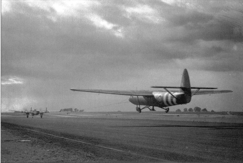
A Horsa glider, which displays the three broad white recognition stripes of the Allies, is towed skywards by an Armstrong Whitworth Albemarle tug aircraft. (Imperial War Museum, H39183)
