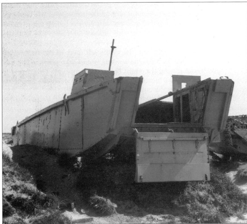
A Derelict Landing Craft Assault (LCA) lying close to the beach many years after the invasion. These wooden vessels, which had a top speed of just six knots and were vulnerable to all types of enemy fire, carried 30 fully loaded troops from the Landing Ships Infantry (LSI) anchored six miles offshore to the beaches. (Ken Ford)
