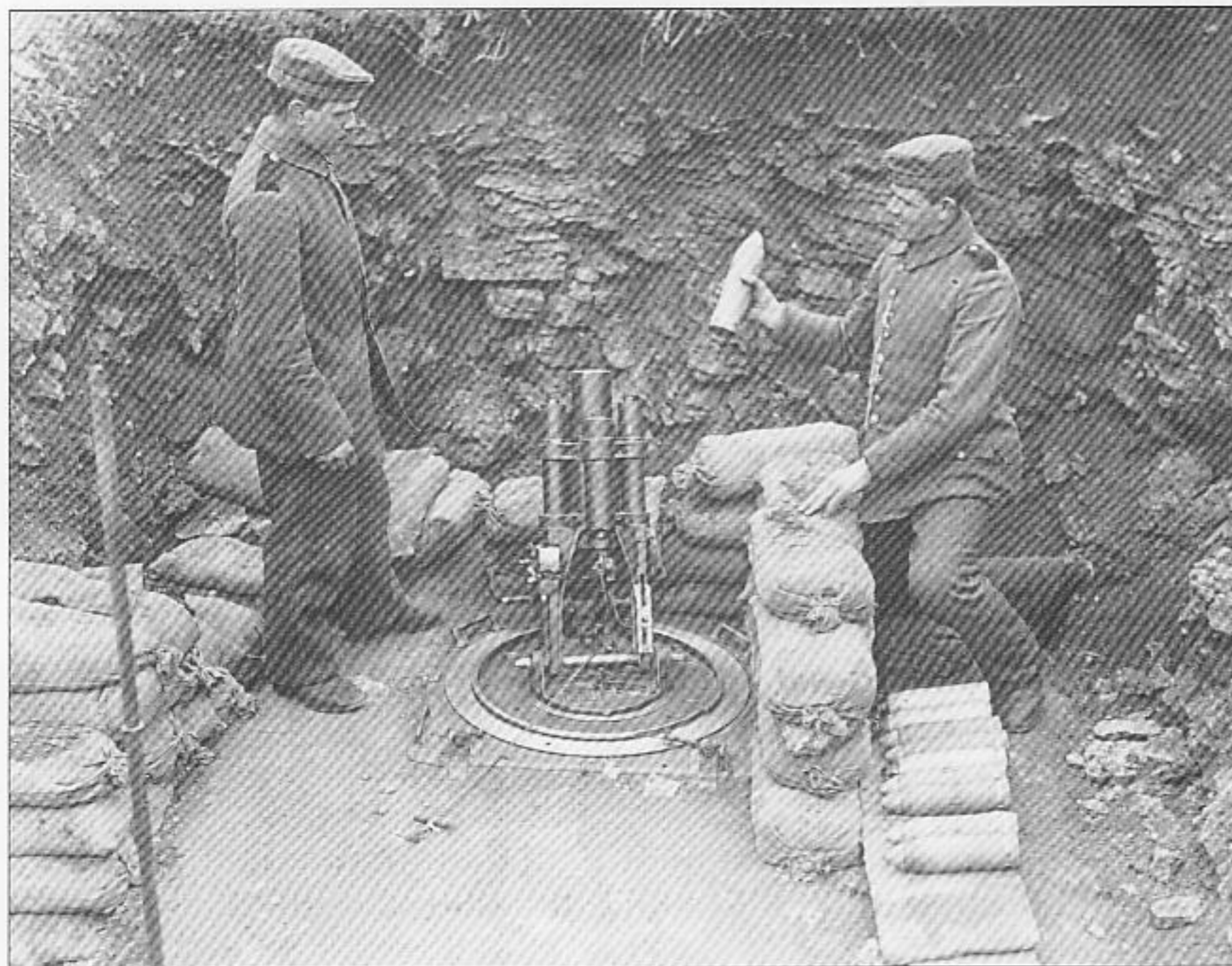
At just over 100 kg (2 cwt) the 'light' 76mm minenwerfer was still a cumbersome beast for mobile infantry operations. Six men could achieve a rate of fire of 20 rounds per minute for short periods. (IWM)
