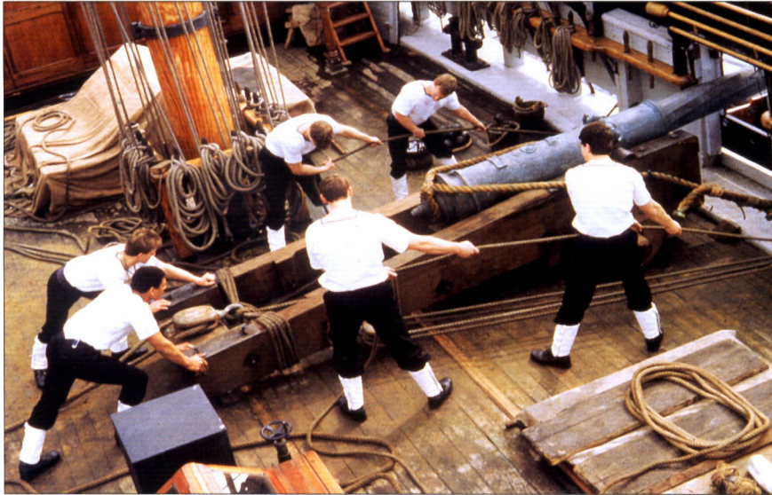
LEFT A Spanish cañon de batir recovered from a Spanish Armada wreck, mounted on a replica Spanish carriage. In 1988 a modern Royal Navy gun team recreated the Spanish gun drill used during the Armada campaign. Here they are dragging the piece back from the gun port to reload it. (Dr Colin Martin)
