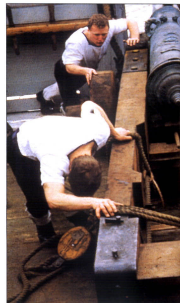
BELOW The same Royal Navy crew have loaded the piece and are now attempting to run it back up to the gunport. Unlike the English four-wheeled truck-carriages, the Spanish relied on these far more cumbersome two-wheeled sea carriages. (Dr Colin Martin)
