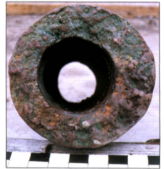
ABOVE A miscast and broken muzzle-end of a media culebrina from El Gran Grifón (now in the collection of the Shetland Museum, Lerwick). The miscast barrel is evidence of the poor quality and hasty production inherent in the Spanish gun-founding programme, which was stretched to the limit to accommodate the ordnance needs of the Armada. (Dr Colin Martin)
