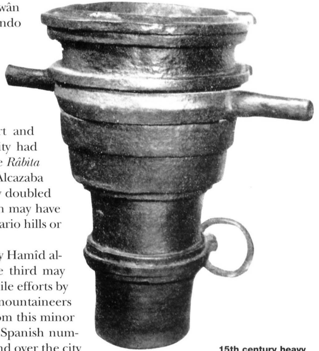
15th century heavy Castilian mortar from Burgos with an early example of trunnions. (Museo del Ejército, Madrid)
