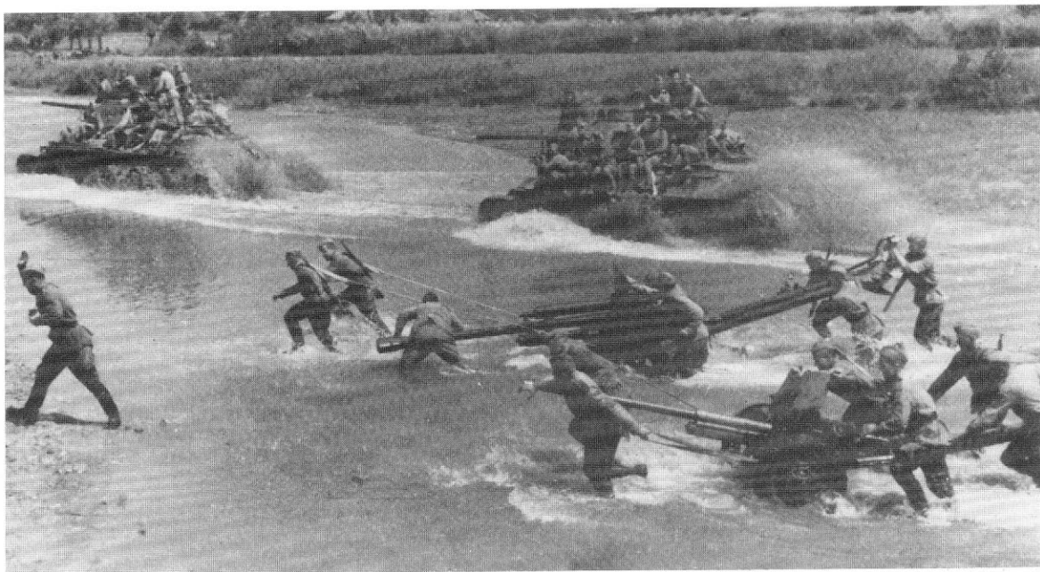
Troops of the 1st Ukrainian Front cross a river on the outskirts of Lvov during the July 1944 fighting. In the foreground, troops manhandle a 45mm Model 1942 anti-tank gun and a ZIS-3 76mm divisional gun; in the background are two T-34 Model 1943 tanks. (Soufot)
