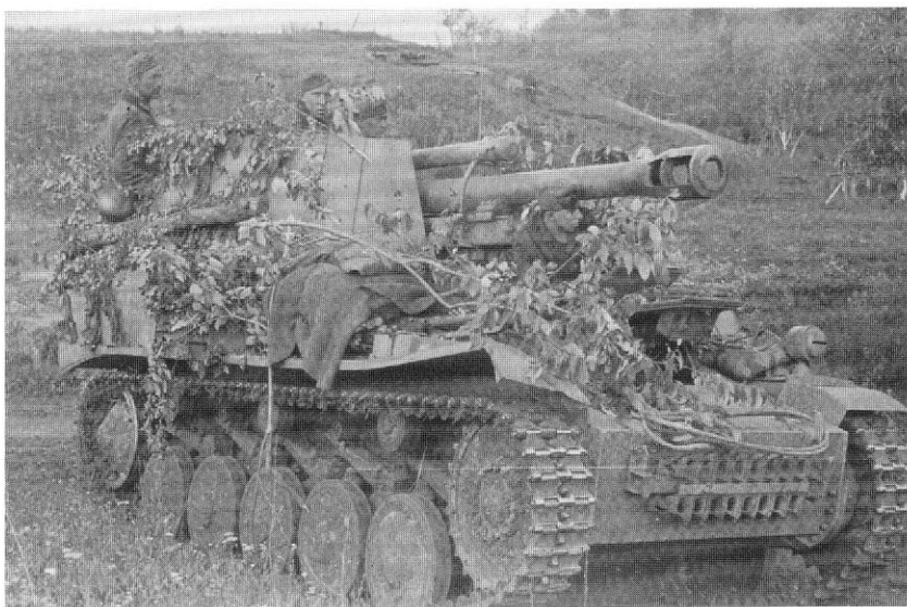
The most common self-propelled howitzer in German service was the 105mm Wespe howitzer, based on the obsolete PzKpfw II tank chassis. This weapon was introduced in the summer of 1944 to replace towed howitzers. The heavy foliage is no doubt due to the threat posed by the Red Air Force at this stage of the war. (National Archives)
