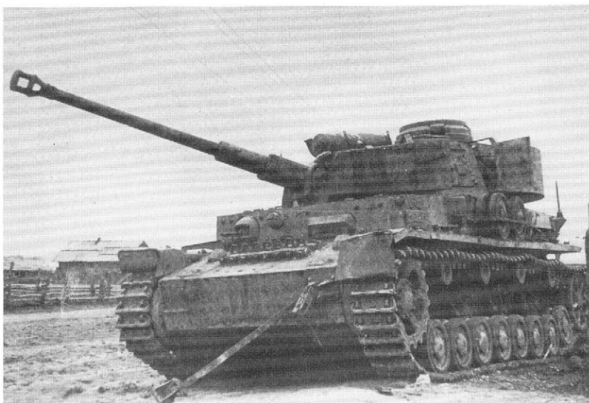
A late production PzKpfw IV Ausf. G with added glacis armour lays abandoned after Operation Bagration. German tank units seldom distinguished the many subvariants of PzKpfw IV tanks, usually referring to these later types with the KwK40 L/48 gun as PzKpfw IV (lang) due to its longer barrel. This type was still an even match with the Soviet T-34 in 1944. (Sovfoto)
