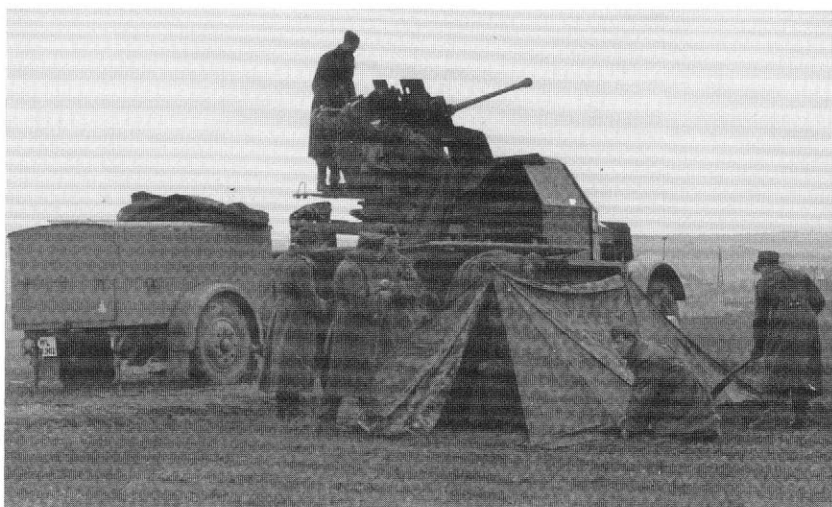
Tactical air defence for Army Group Centre was provided by a variety of weapons including the 37mm FlaK 36, seen here carried on the Krauss Maffei 8-ton SdKfz 7/1 half-track. These were generally issued to special Luftwaffe air defence units rather than Wehrmacht units.
