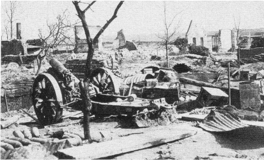
◀ A captured British 6in 26cwt howitzer position with fuzed ammunition and sandbagged dugouts or shelter tarpaulins. Ludendorff captured 147 such weapons in his 1918 offensives. The 6in, designed in 1915, was the BEF's standard and effective medium howitzer. It had a range of 11,600 yards (6.5 miles) with a 100lb shell. Fifth Army began with 262 such howitzers and Third Army had 217. (IWM Q29971)
