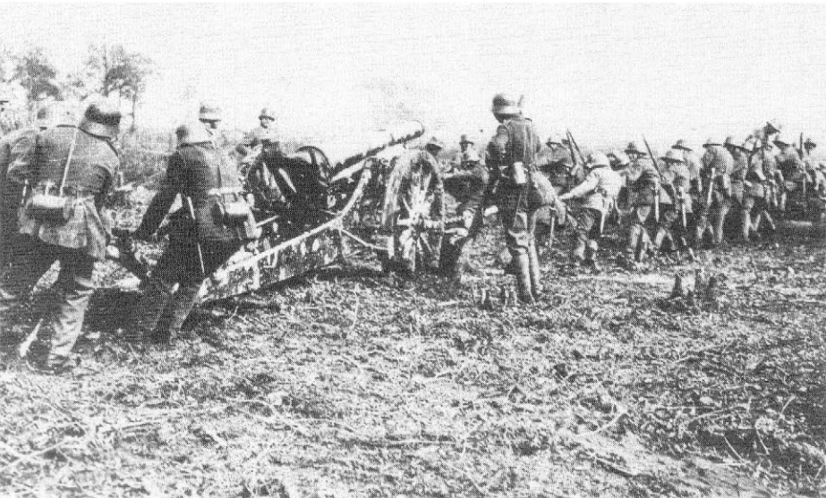
◀ German artillerymen manhandle forward a Model 1913 130mm heavy field gun, probably in the Somme region. The gun weighed 5.7 tons and fired an 891b shell to a range of nearly 15,750 yards (9 miles). Rate of fire was two rounds a minute and maximum elevation 26°. Seventeenth and Second Armies had 39 of these pieces organized in two-gun batteries. (IWM Q56559)
