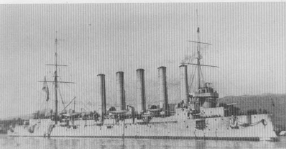
◀ The Russian cruiser Askold, completed 1903, armed with twelve 6in, twelve 12pdr, eight 3pdr and two 1pdr guns.
