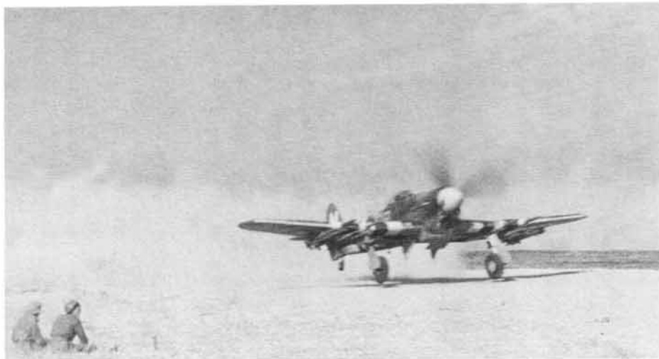
An RAF or RCAF Typhoon (squadron not identified) takes off from a temporary landing strip in Normandy, early July. Note the four rockets slung under each wing. The black and white 'invasion stripes' at the wing roots were painted on to all Allied aircraft involved in the Battle of Normandy as a recognition device. Their presence is often a useful check of the authenticity of film or photographs of the battle. (IWM photograph CL147)
