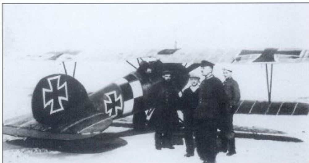
A useful rear view of Sachsenberg's Albatros D Va at MFJ I. This perspective illustrates the five-colour printed camouflage fabric on the wings and tailplane (J Rhyheul)
