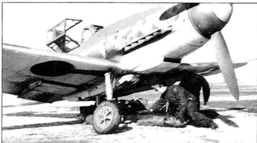
Mechanics prepare an ETC 50/VII rack and 250 kg bombs prior to this Bf 109F-4/B being sent out on its next mission in late 1942. Many of the Hungarian pilots who flew the F-model Messerschmitt on fighter-bomber operations found it easier to handle than their colleagues who used it solely as an interceptor (Petrick)
