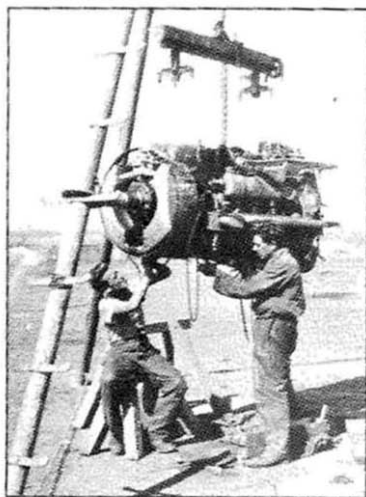
Mechanics work on a DB 605 engine hoisted up by a tripod crane (Punka Archiv)
