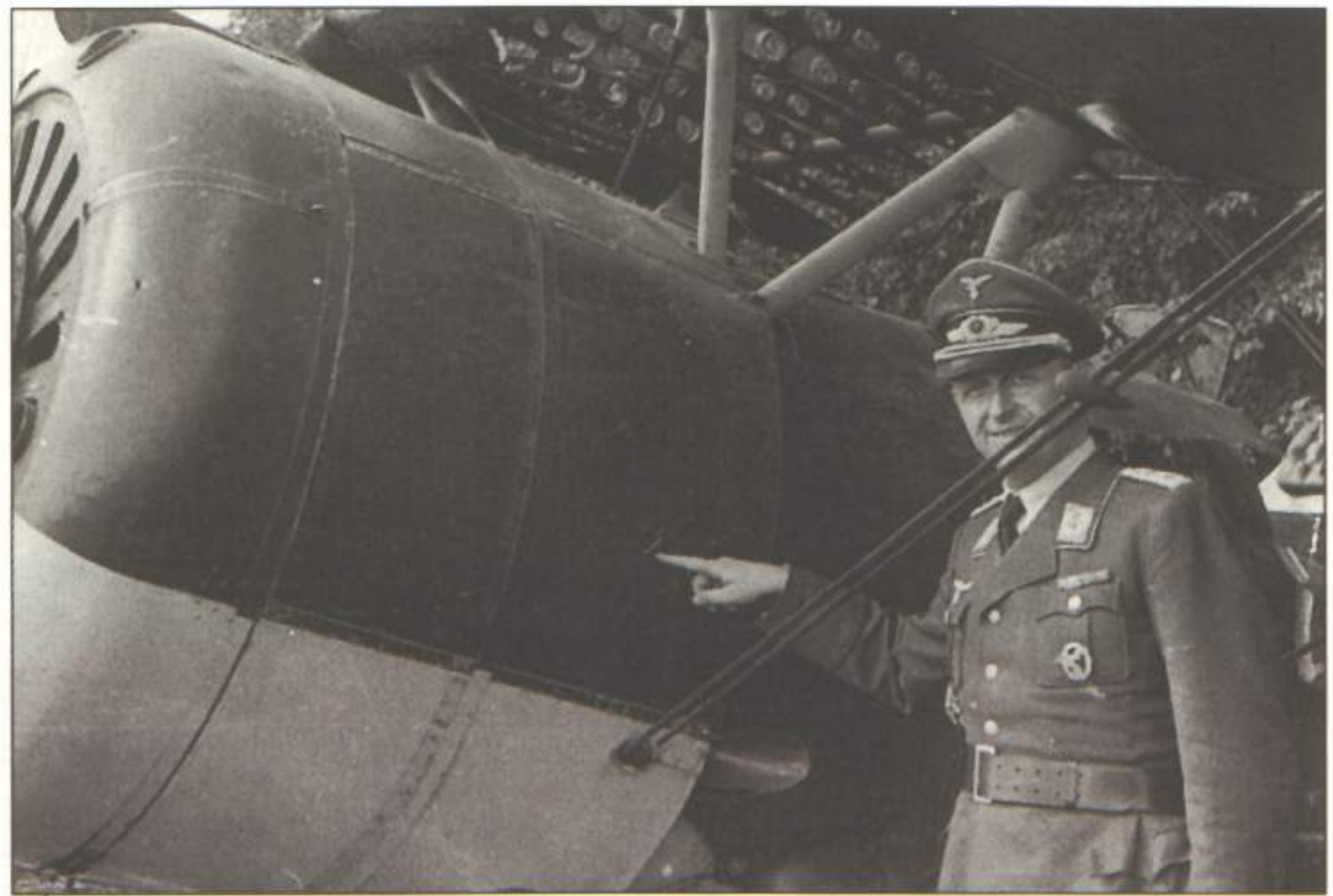
A captured I-152 is examined by a Luftwaffe officer, who points out the hole made by shrapnel, or perhaps a machine gun bullet, to the cameraman (BAK Loc 290)
