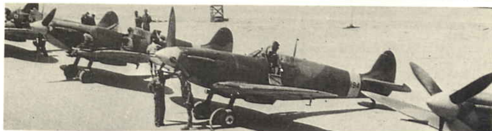
Mk. Vb's in Russian markings await collection at Abadan, April 1943. All in green / grey camouflage, first aircraft is AD194 built at Castle Bromwich in the autumn of 1941. (E23982 IWM)
