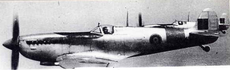
Mk. IX's of the Operational Training Unit, Brusthem, Belgian Air Force. Bare metal finish with black anti-glare panel, yellow fuselage and wing bands. Blue outline to national insignia. (via M. C. Terlinden)
