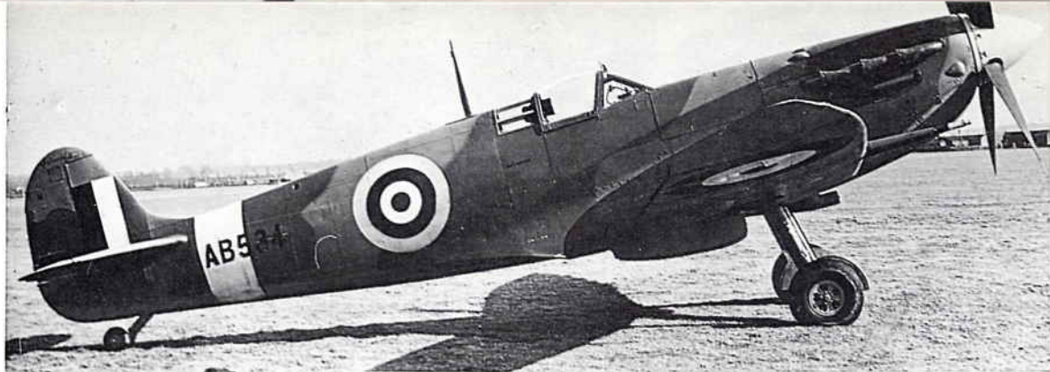
One of the less successful, and not so popular Spitfires was the Mk. VI. Note cabin pressurisation intake and extra frame on canopy, AB534 was later flown on No. 616 'South Yorkshire' Squadron in 1942 by 'Johnnie' Johnson. (HU2195 IWM)
