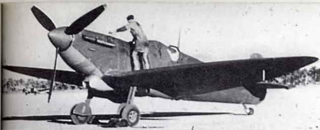
This PR IV was extensively modified by No. 103 MU at Abouqir, Egypt, in the winter of 1942-43. Its apparently ragged appearance is the result of much sealing and sanding to give a smooth finish. Fitted with locally made pointed wing tips, a highly tuned engine and Abouqir type filter, it was one of several later used by No. 680 Squadron for long range sorties over Salonika. (T. P. M. Cooper-Slipper)
