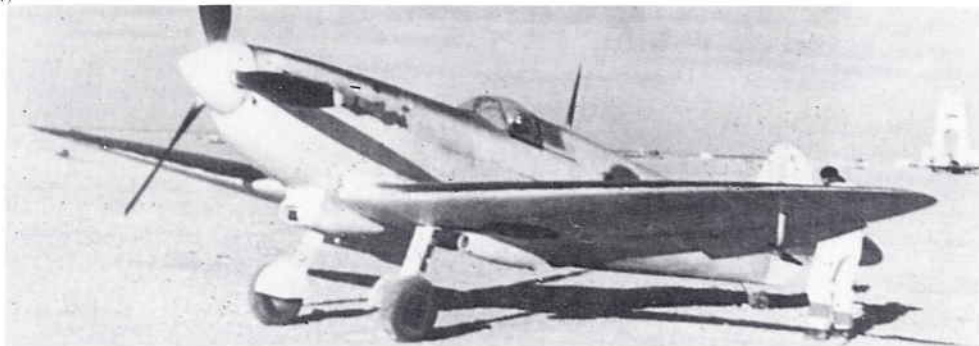
This PR IV was extensively modified by No. 103 MU at Abouqir, Egypt, in the winter of 1942-43. Its apparently ragged appearance is the result of much sealing and sanding to give a smooth finish. Fitted with locally made pointed wing tips, a highly tuned engine and Abouqir type filter, it was one of several later used by No. 680 Squadron for long range sorties over Salonika. (T. P. M. Cooper-Slipper)
