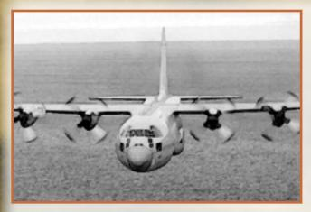
C-130 has proven itself a hardy combat air transport since its introduction. Variants of the C-130 were used in roles ranging from medical evacuation (the HC-130), to special operations insertion and extraction (the MC-130), to weather flights into hurricanes and cyclones (the WC-130), to combat against ground forces (the AC-130, detailed above). The C-130 is capable of carrying 92 soldiers, 64 fully equipped paratroopers (who sit facing one another and are
