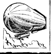
Military airships use helium; civilian "zeps" use hydrogen. In both types, the gasbag is divided into small cells, so that even a large number of punctures will leave the ship serviceable. The hydrogen-filled airships also incorporate a halon fire-extinguishing system and flameproof materials in the gasbag.
