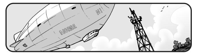
Nearly all rigid airships carried their framework inside the hull, but one was successfully flown for more than a decade with an exterior aluminum covering (see ZMC-2, p. 97).
