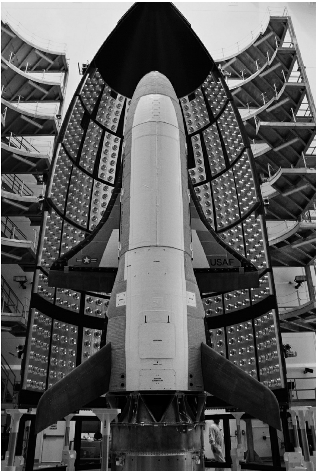
The X-37B unmanned space-plane being prepared for launch inside a fairing nosecone. The MQ-14 Lunar Hawk attack drone is launched in an identical manner. (NASA)
