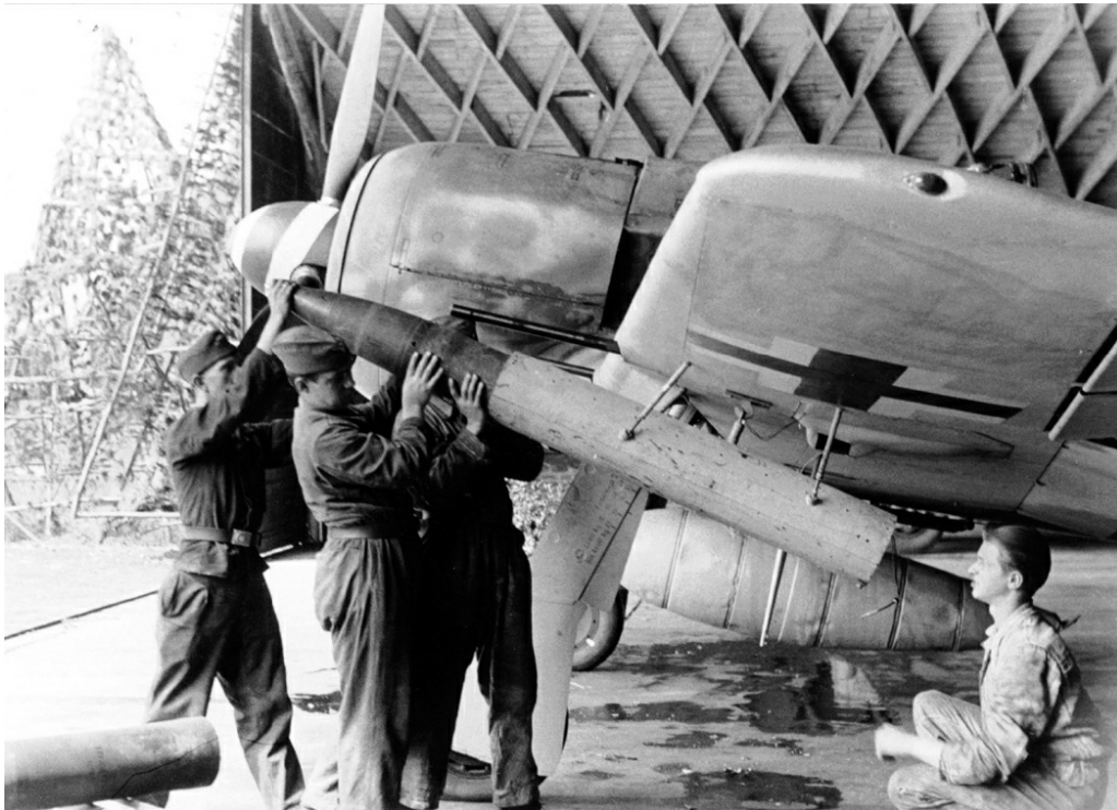
A Werfer-Granate 21 rocket being loaded onto a Focke-Wulf Fw 194 fighter. Luftwaffe pilots disliked the drag caused by the launch tubes, but this weapon proved very effective during Operation Lyre . (Bundesarchiv Bild 101I-674-7772-13A)
