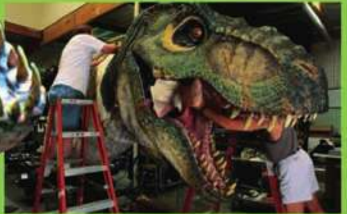
▲ KILLER JAWS Teeth are glued to the jaws, the mouth is lined with flesh-coloured latex, and flexible skin is wrapped around the steel skull.
