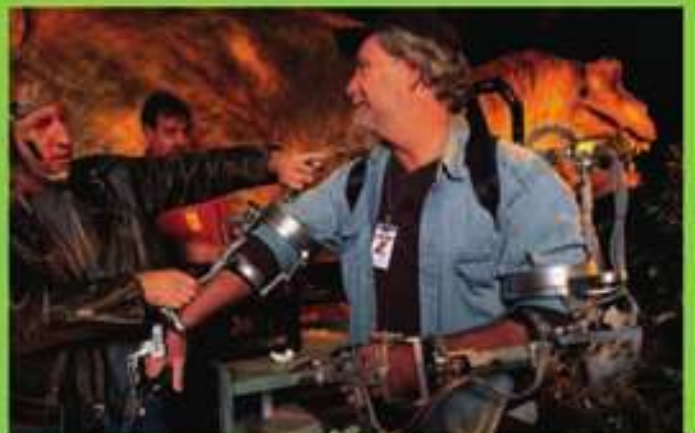
▲ PUPPET MASTER The dinosaur's movements are controlled by a “telemetry suit” worn by an operator. This suit controls the arms.
