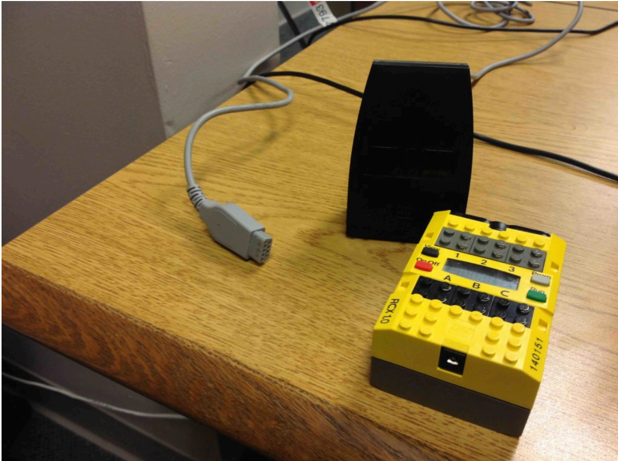
Figure 1. Lego RCX brick and IR transceiver.
