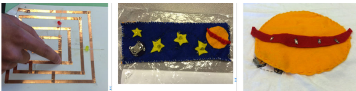
Figure 7. Annie’s three e-textile projects from left to right: paper circuit (maze), starry bracelet, and glowing planet with hidden microcontroller (lower left of picture).
