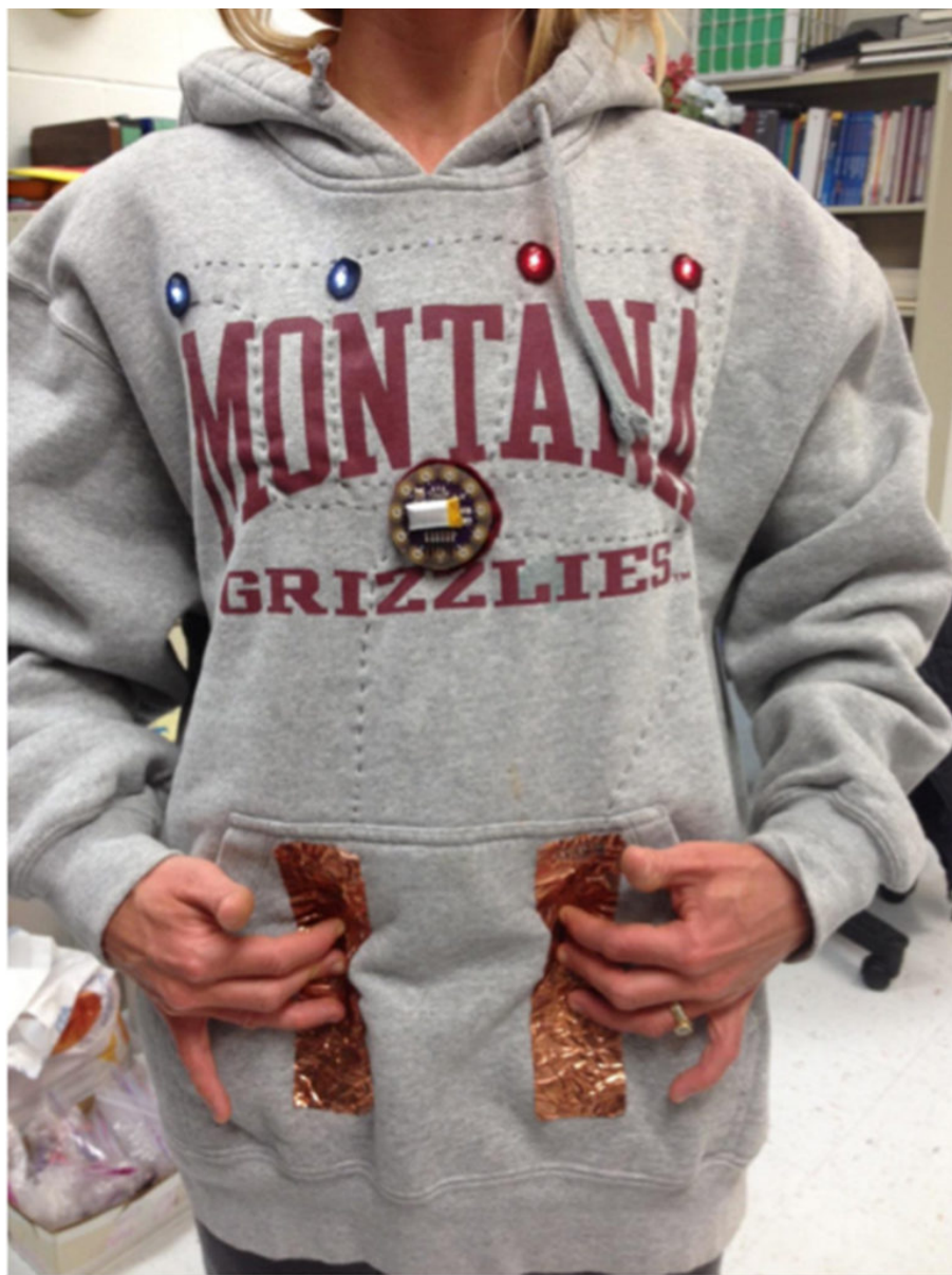
Figure 1. James Howell's programmable human sensor hoodie.
