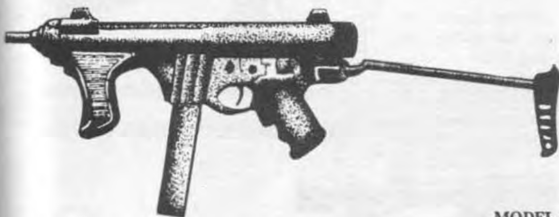
MODEL 12 BARETTA SUBMACHINE GUN: — Weight: 8lb 5oz (3.77kg) fully loaded. Length: 25" (645mm), 16.5" (418mm) with stock folded. Round: 9mm parabellum. Rate of Fire: rounds rounds per minute. Nation of Manufacture: Italy.
