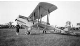
Western Australian Airways de Havilland DH50 at Maylands airfield. Passengers ride in a compartment under the top wing, in front of the pilot
