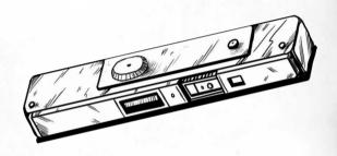
A more foolproof solution is to use a rollover camera, which requires no special skill to operate. These special devices are small boxes that fit within the palm of the hand. As the name suggests, they are designed to be rolled over documents, exposing a moving strip of film. The camera has an internal light source, making it entirely self contained. A single roll of film may be used to photograph up to 100 documents.
